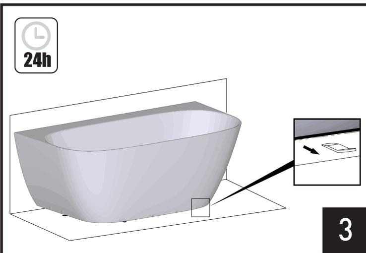
After removing bathtub spacers, apply silicone sealant (not provided) in the gap. Wait **24 hours** for fully sealed. Installation complete.
