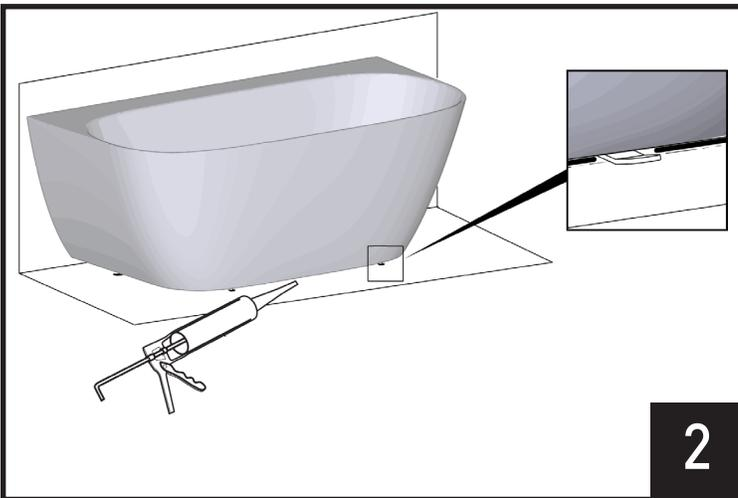
Apply silicone sealant along bathtub edge footer. Do not seal over bathtub spacers.
