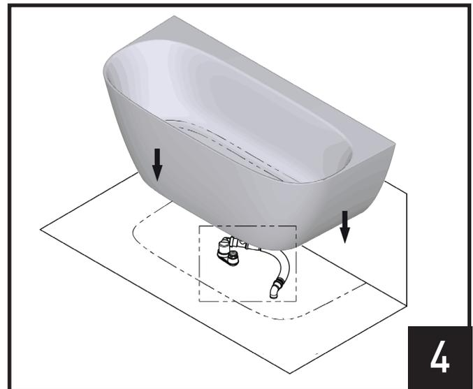
Install bathtub K36/K40 waste drain into floor surface. Install bathtub and align drain with floor waste drain.
