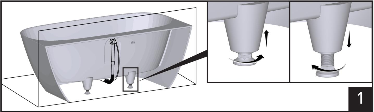
To adjust and level the bathtub, either raise or lower by rotating the bathtub feet as needed.
