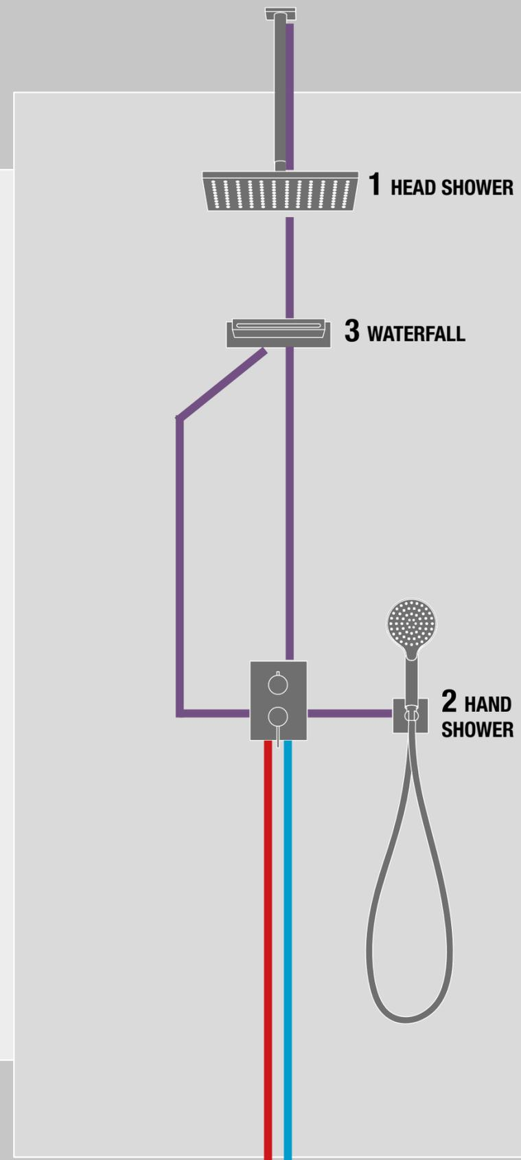
**T<sub>38°</sub>** TERMOSTATICO | THERMOSTATIC
